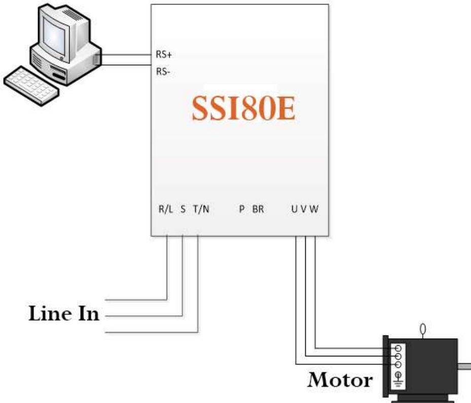
When using communication to control the drive, you can set the frequency directly by writing register 10000 . The register value is in the range of 0.00 ~ P5-08, unit 0.01Hz.
